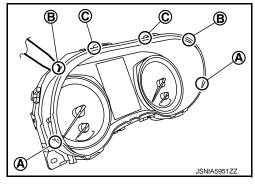
4. Pull the front cover straight to remove it from the unified meter control unit.
