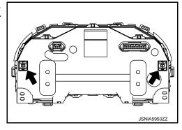
5. Disconnect the harness connector and remove the combination meter.
